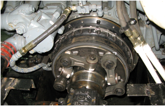
Fig. 12 Overview of Centa company's flexible coupling B with flexible link
