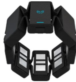
Fig. 1 MYO, EMG measurement device
