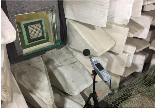
Fig. 8 Receiver (full anechoic chamber) room
