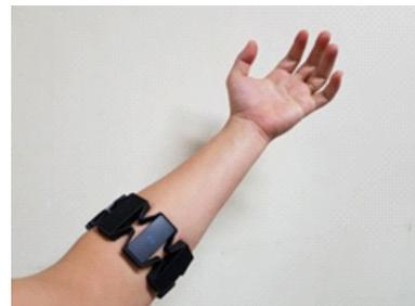
Fig. 2 Photograph of worn EMG measurement device
