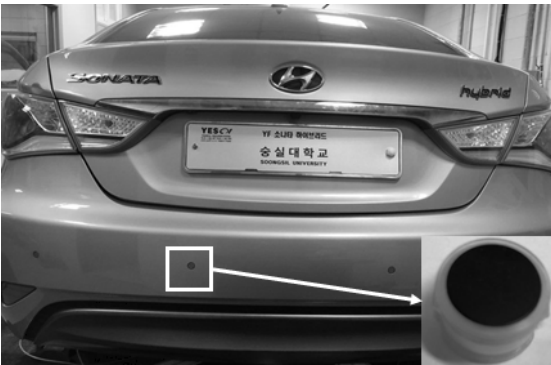
Fig. 1 Ultrasonic sensors on a bumper
