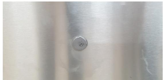
Fig. 4 Target disk located at the impact point
