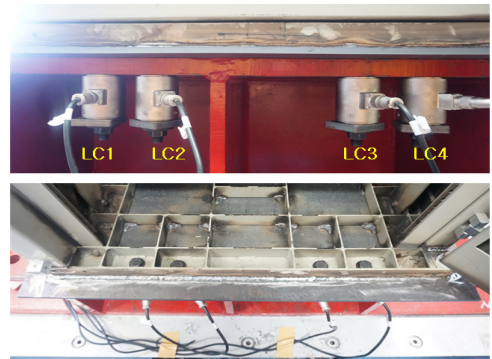
Fig. 4 Anchor bolt with ring type load cell
