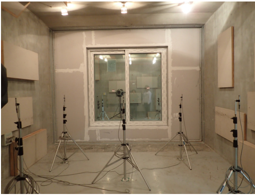
Fig. 3 Sound insulation performance measurement set-up
