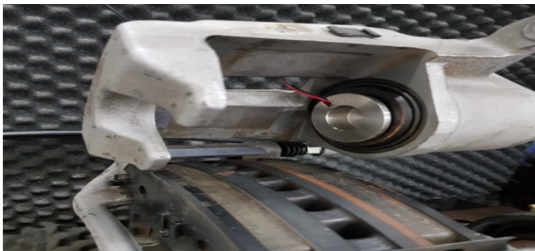
Fig. 6 Brake caliper with pzt module
