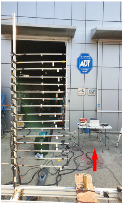
Fig. 12 Photograph of near-field measurement for supersonic free-jet
