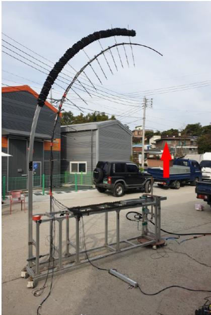
Fig. 14 Photograph of far-field measurement for supersonic free-jet
