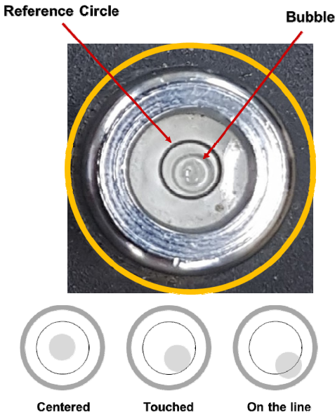
Fig. 9 Horizontal level indicator of the accelerometer (Kinematics ES-T)
