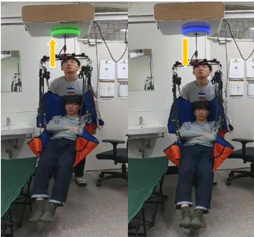
Fig. 18 Experiment for force control mode
