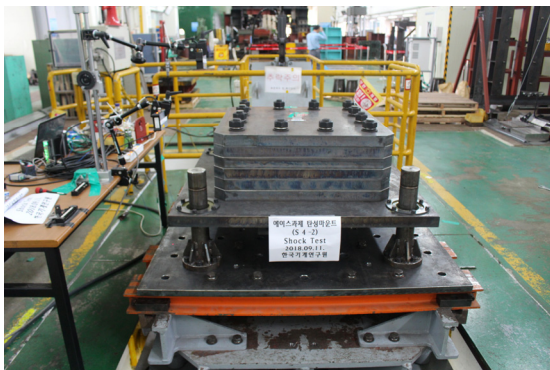
Fig. 5 Shock test with one mount in vertical direction
