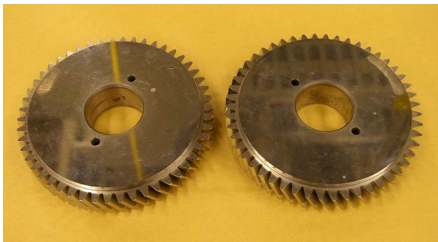
Fig. 6 The test helical gear pair used in the previous study
