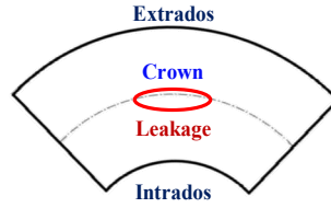
Fig. 12 Elbow with a through crack
