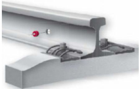
Fig. 3 Sensor installation example
