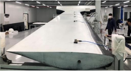
Fig. 12 Modal test of the main wing
