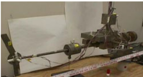
(a) 5.5% scaled dynamic model for AH-1G
