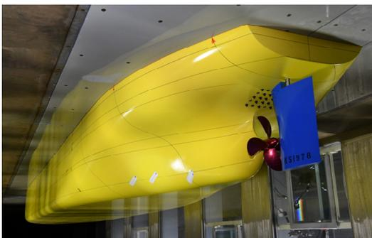
**Fig. 16** Model ship setup for application test of sensor array
