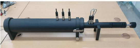
Fig. 8 The impedance tube for measuring 29absorption coefficient
