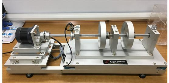
Fig. 5 Rotor-kit system with 3 bearings
