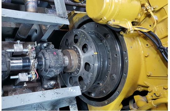
**Fig. 16** Overview of Stromag company's flexible coupling C
