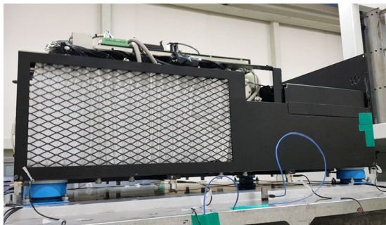
Fig. 5 Fuel cell power pack vibration test
