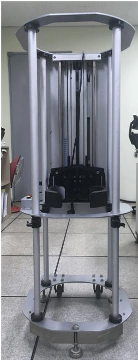
Fig. 1 Rubber ball dropping machine
