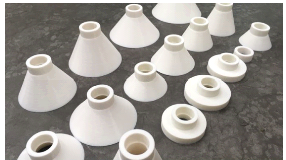
Fig. 14 Horn guide specimens made by a 3D printer
