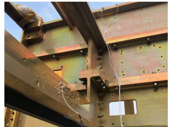
Fig. 10 Accelerometer location of the DTRM surface
