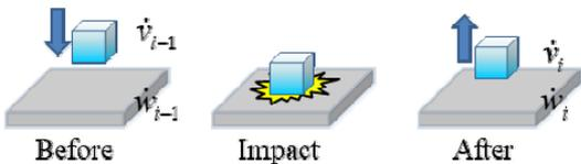
(b) Impact mechanism between impact damper and beam element
