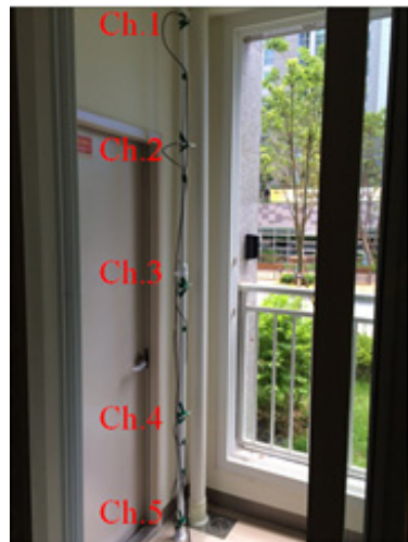
Fig. 3 Microphone measurement point
