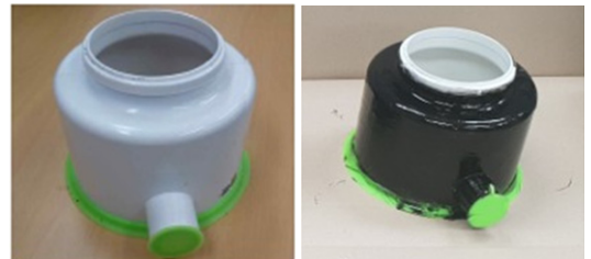
Fig. 5 Existing commercial products (left) and rubber-paint reinforcement status (right)
