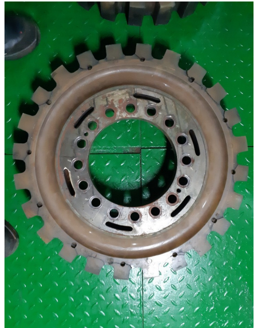
Fig. 18 Damaged flexible coupling on the model C
