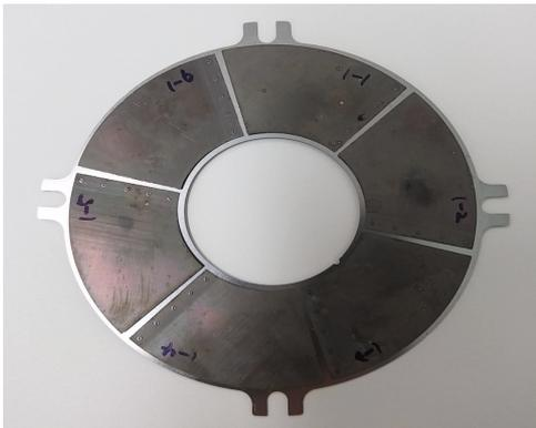
Fig. 1 Air foil thrust bearing for FCEV
