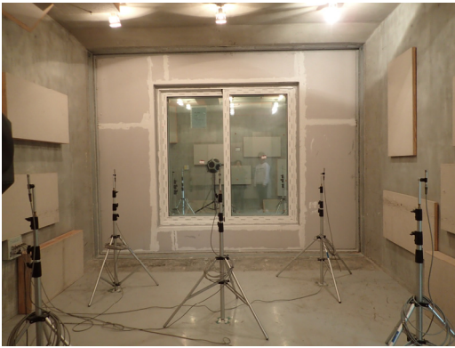
Fig. 3 Sound insulation performance measurement set-up
