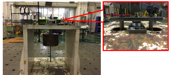
Fig. 6 Load-deflection measurements for representative wire mesh mount prototypes
