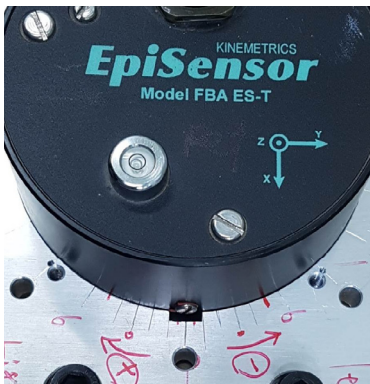
Fig. 7 Setup to change the direction alignment of accelerometer
