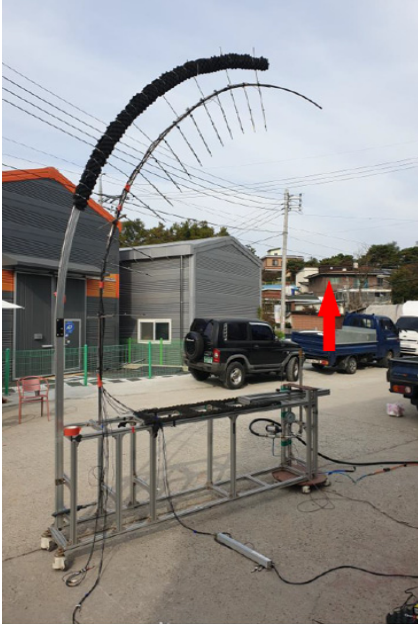
Fig. 14 Photograph of far-field measurement for supersonic free-jet
