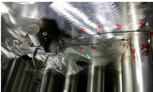
Fig. 3 Strain gages and accelerometer installed on CEA guide tube and UGS support plate
