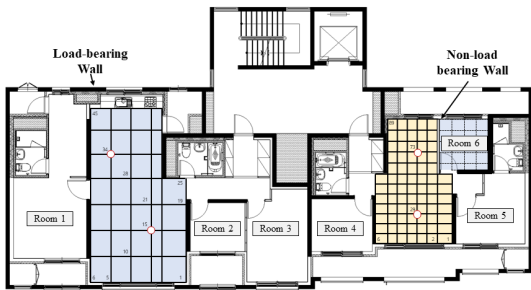
Fig. 4 Experimental set-up to measure vibration characteristic of floor structure
