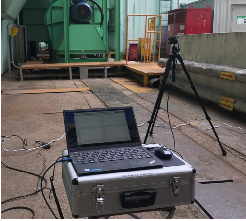
Fig. 15 Experimental setup for vibration extension of field motor
