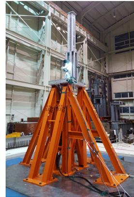
Fig. 13 Photo of seismic test jig with BMCARDM
