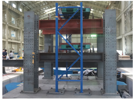
Fig. 14 Sliding of pallets after EQ 300 % test
