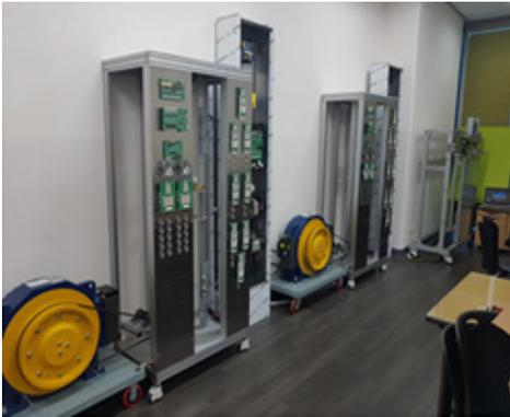
**Fig. 14** Lift simulator sets
