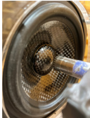
(b) Microphone and speaker for near field sound measurement at low frequency
