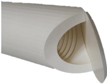
Fig. 9 Waveguide specimen made by a 3D printer
