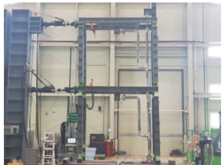
Fig. 4 Side sway test of the riser pipe with pressure joints
