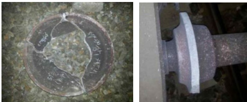
Fig. 1 Case of accident due to wheel broken
