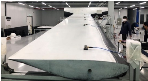
Fig. 12 Modal test of the main wing
