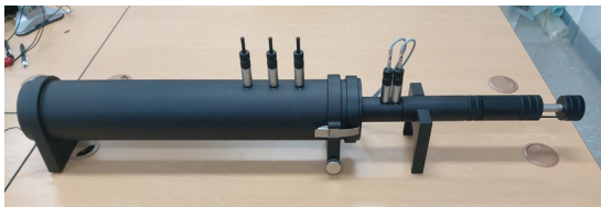
Fig. 8 The impedance tube for measuring 29absorption coefficient
