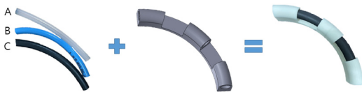
Fig. 8 Combination of a waveguide tube and a supporter (A : silicon, B : PVC, C : EPDM)
