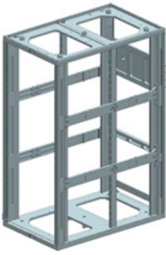
Fig. 6 Configuration of finite element mode of body frame
