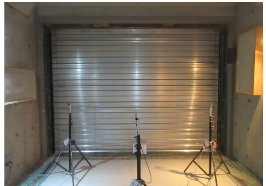
Fig. 7 Specimen installation for sound insulation test
