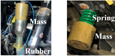
(a) Base frequency DVA composed of rubber-mass (b) Peak frequency DVA composed of spring-mass
