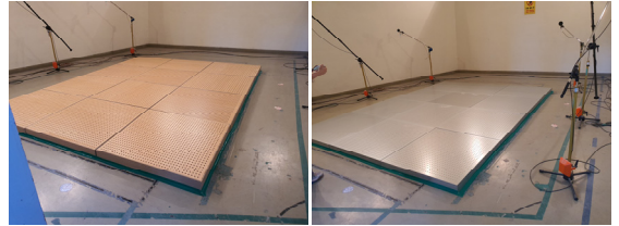
Fig. 3 Measurement of sound absorption coefficient in reverberation room
