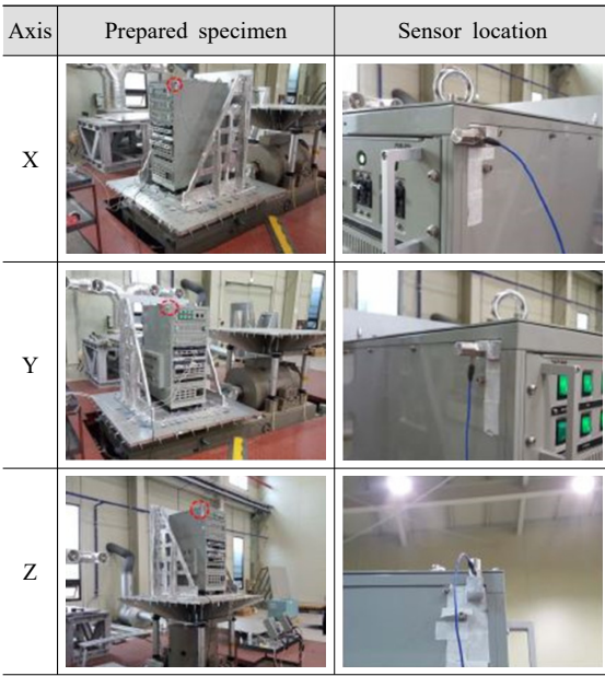
Fig. 12 Configuration of vibration test of EER system
