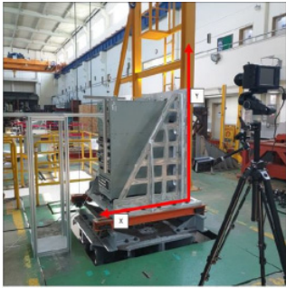
Fig. 14 Measurement of dynamic displacement under shock
