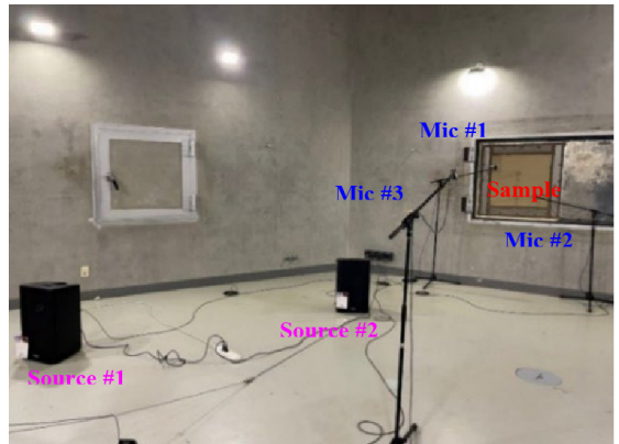
Fig. 4 Reverberant room with experimental equipment
