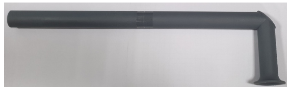
Fig. 9 Prototype of ‘L’ shape waveguide coupled with a horn guide
