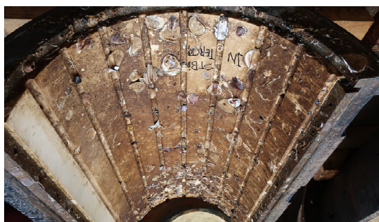
Fig. 12 Barnacle generated in the upper bearing of the inter strut
