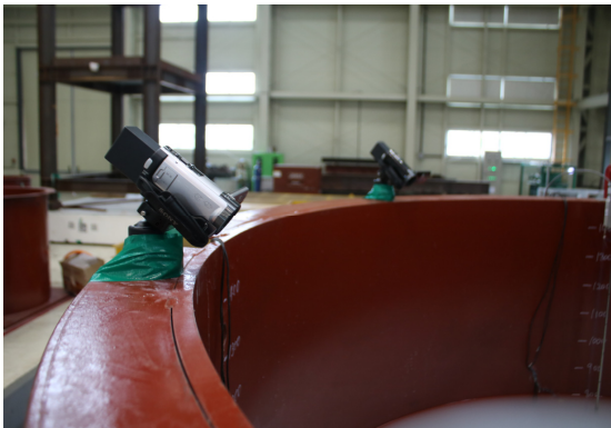
Fig. 5 Installed digital camcorder
