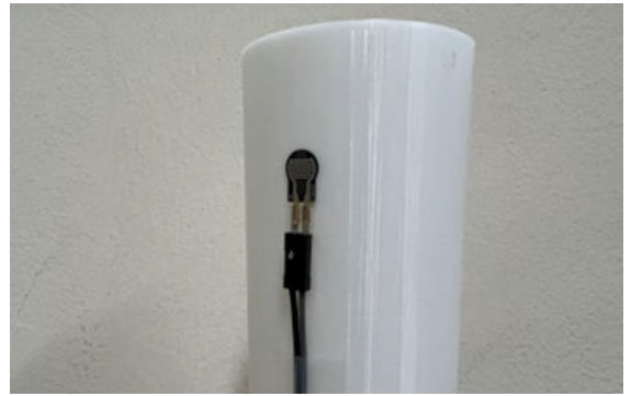
Fig. 8 Pressure sensor located on object surface
